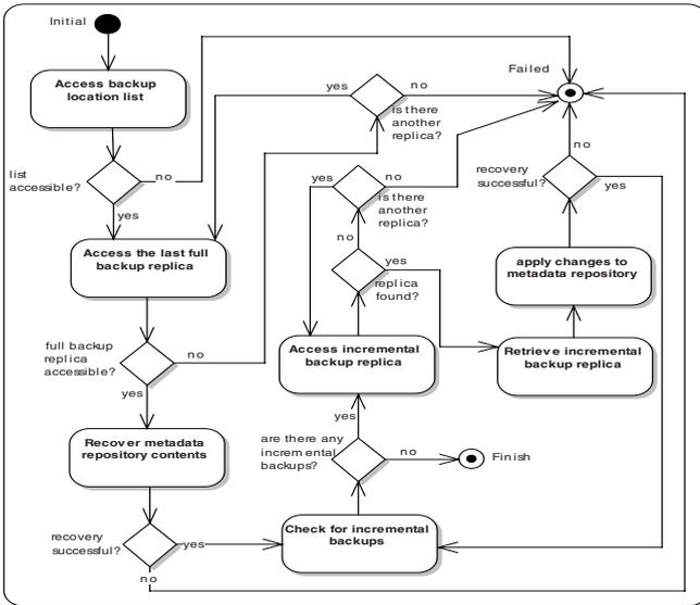
Fig. 2. High-level activity diagram of the Recovery service
