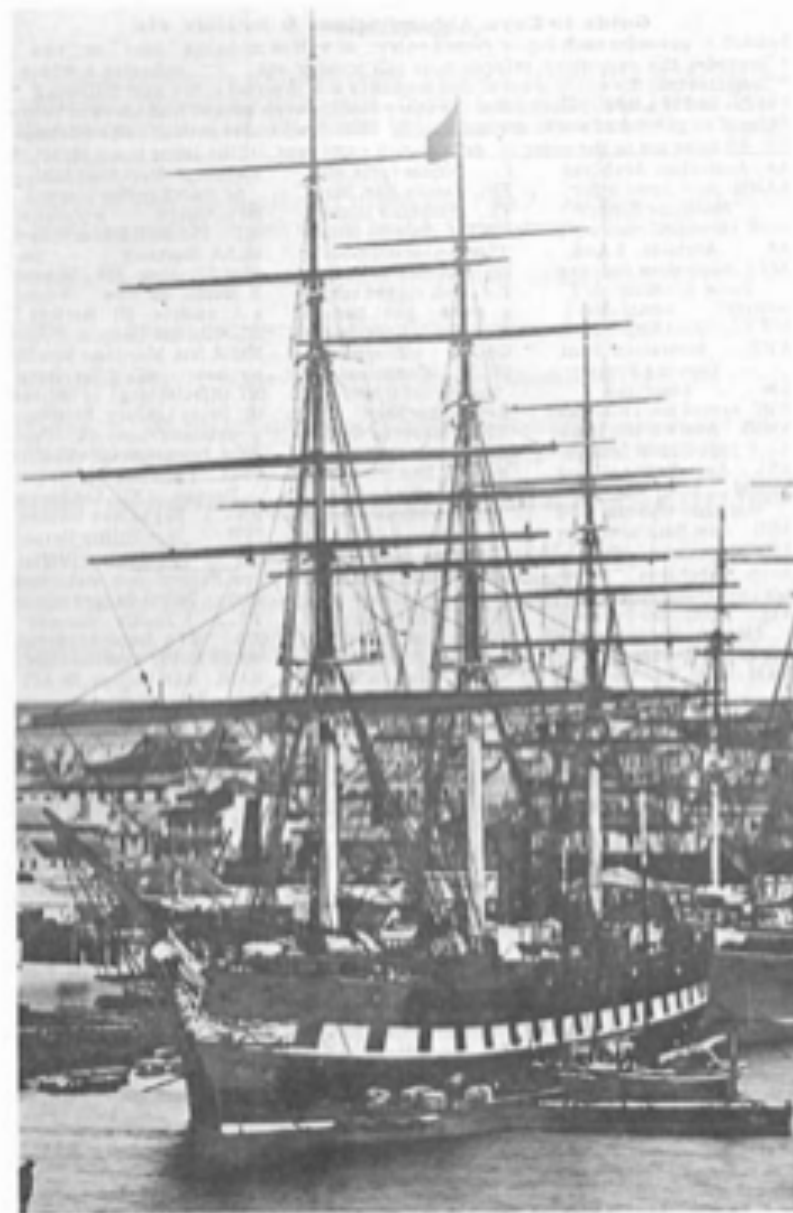
The famous auxiliary ship Great Britain , of 3343 tons, at Circular Quay, Sydney, 1886. She was the first iron screw steamer in the world and was designed to carry over 600 passengers. On the England-Australia run from 1852 to 1876, she probably brought more settlers to Australia than any other ship. Photo from the author's collection. (See further illustration on page 21-6).
