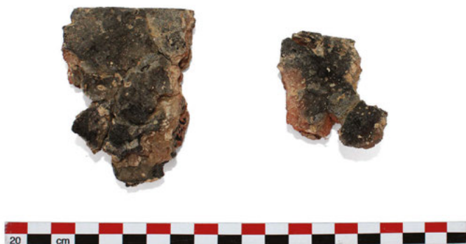
Figure 4. Furnace rim (Inv. KIT 939) showing evidence of reducing firing conditions and a thin layer of slag.
