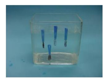
Figure 2. How weights of the diver influence floating if the volume is approximately constant.
