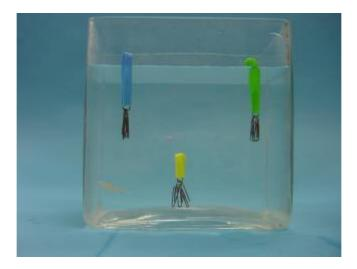
Figure 3. How volume influences the floating if the mass does not change significantly.
