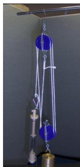
Figure 1. Equipment for physical pulley experiment.
