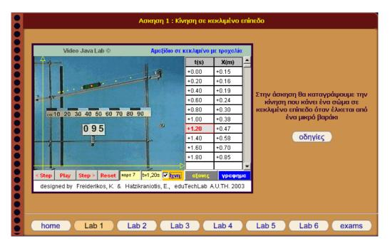
Figure 2: Typical screenshot of a lab activity in VJL (Lab-1). Students take measurements for the motion of a cart on inclined plane.
