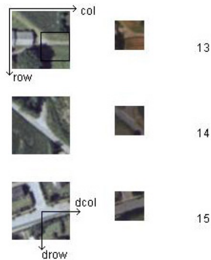
Fig. 2 Patches of the aerial image and the orthoimage are matched and pixel coordinates (drow, dcol) will be found at the position of best fit.
