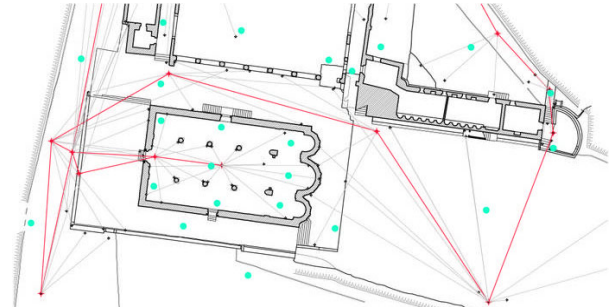
Figure 2: Positioning of Scanworlds (blue) and station points (red) for the internal and external acquisitions.
