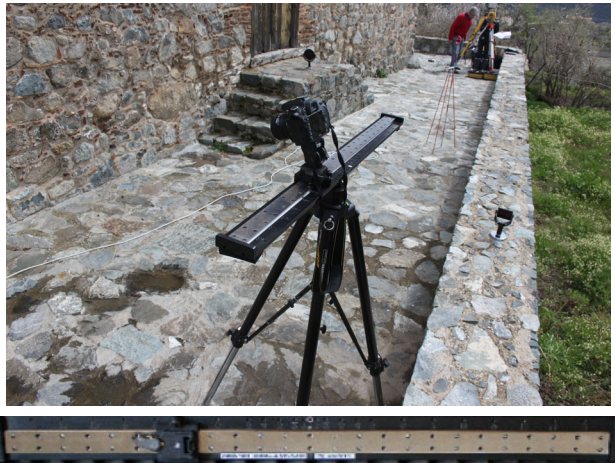
Figure 4: The typical setup of the ZScan and the slide bar
