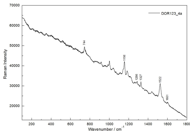
Figure 6: Raman spectrum obtained on a green area of sample DOR123.
