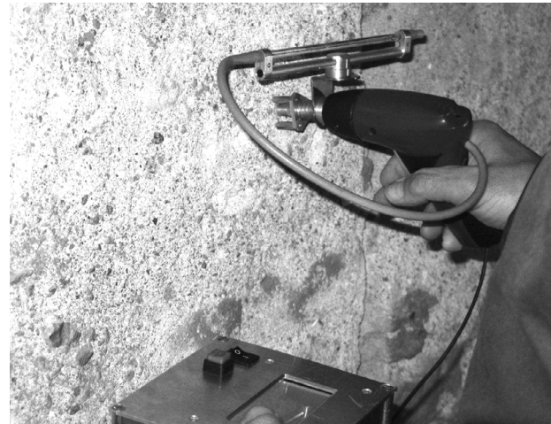
Figure 4. Application of a microtube device for in situ measurement of mortar water absorption characteristics.
