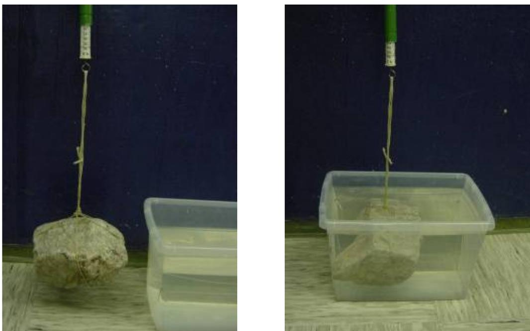
Figure 4. Measuring the weight (left) and apparent weight (right) of the rock.
