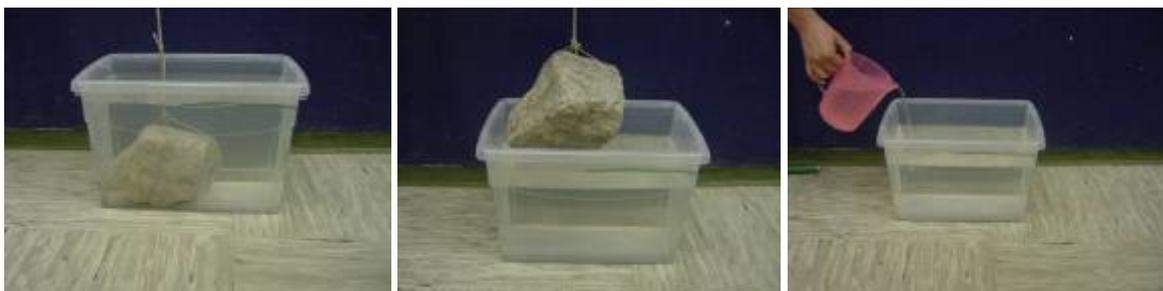
Figure 5. When the rock is submerged the water level rises and the level of the water is marked on the container. How much water should be added to reach the marked level?
