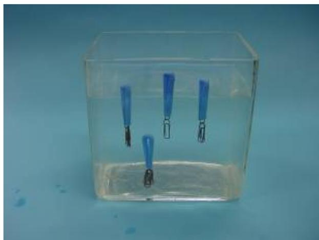
Figure 2. How weights of the diver influence floating if the volume is approximately constant.
