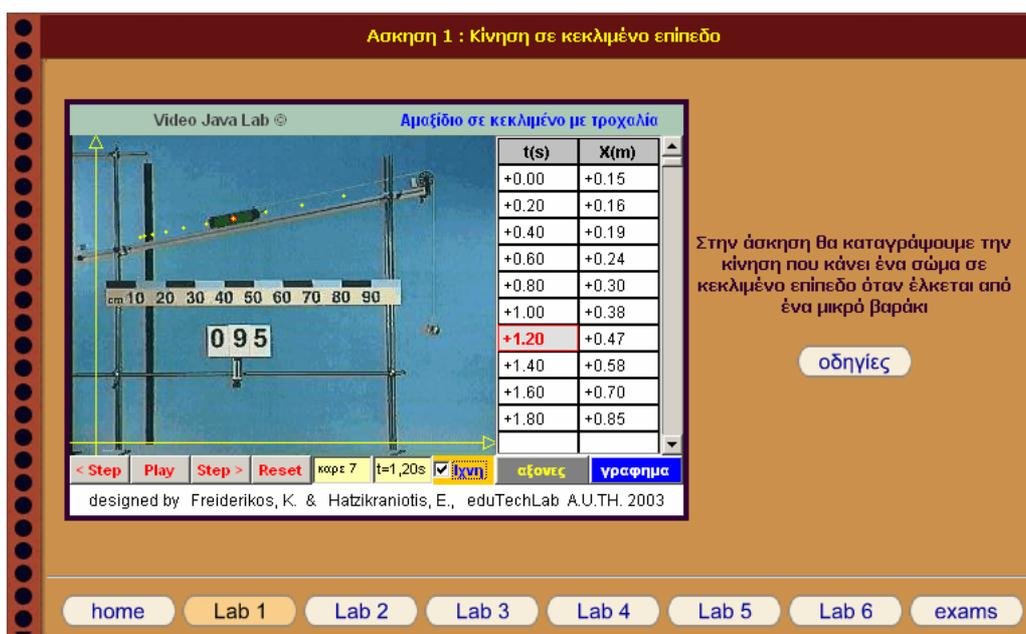
Figure 2: Typical screenshot of a lab activity in VJL (Lab-1). Students take measurements for the motion of a cart on inclined plane.
