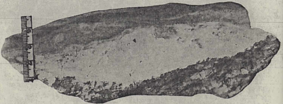
Plate III. Havara from Kalopsida area showing slight banding and concretions and hard Kafkalla on top. Scale in centimetres (cms).
