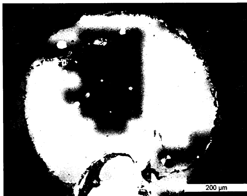
b: Micrograph of a piece of slag with a large globular matte inclusion. It contains metallic iron (bright drops) and slightly more metallic copper (in the cracks and at the periphery).
